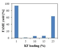
**Figure 9** Effect of different KF loading on eggshell on biodiesel yield. Reaction conditions: reaction temperature 50°C, catalyst amount 5 wt%, molar ratio of methanol to oil 6:1 and 1 hour of reaction time.
