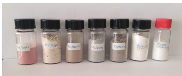
Figure 1 Prepared ZSM-5 samples with different promoters
