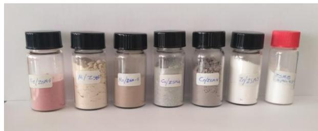
Figure 1 Prepared ZSM-5 samples with different promoters
