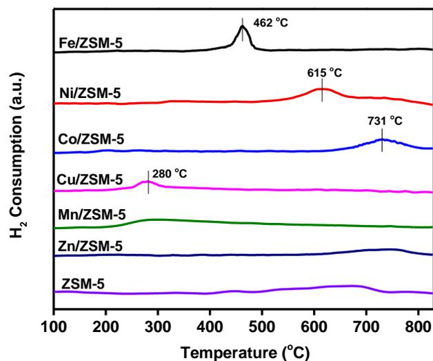
Figure 6 H<sub>2</sub>-TPR profiles of the catalysts
