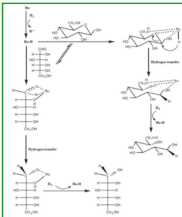
Scheme 4: Mechanism of glucose hydrogenation over Ru/MCM41 [30].
