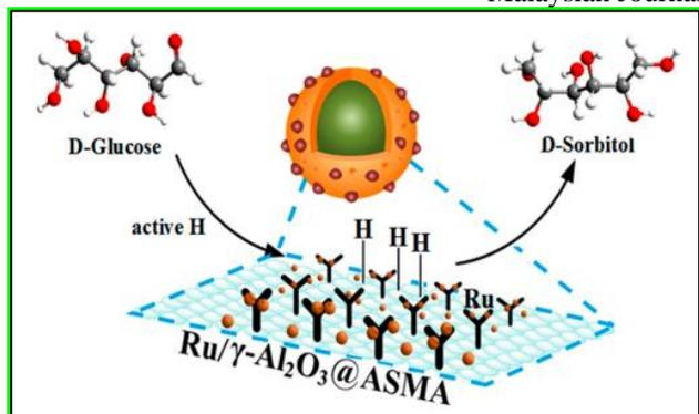
Scheme 5: The hydrogenation route from glucose to sorbitol using 5%Ru/γ-Al<sub>2</sub>O<sub>3</sub>@ASMA pellet as catalyst [2].
